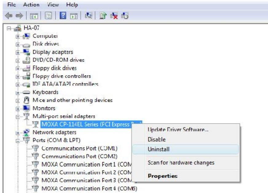
2. Select **Delete the driver software for this device** and click **OK** to proceed with uninstalling the board.
