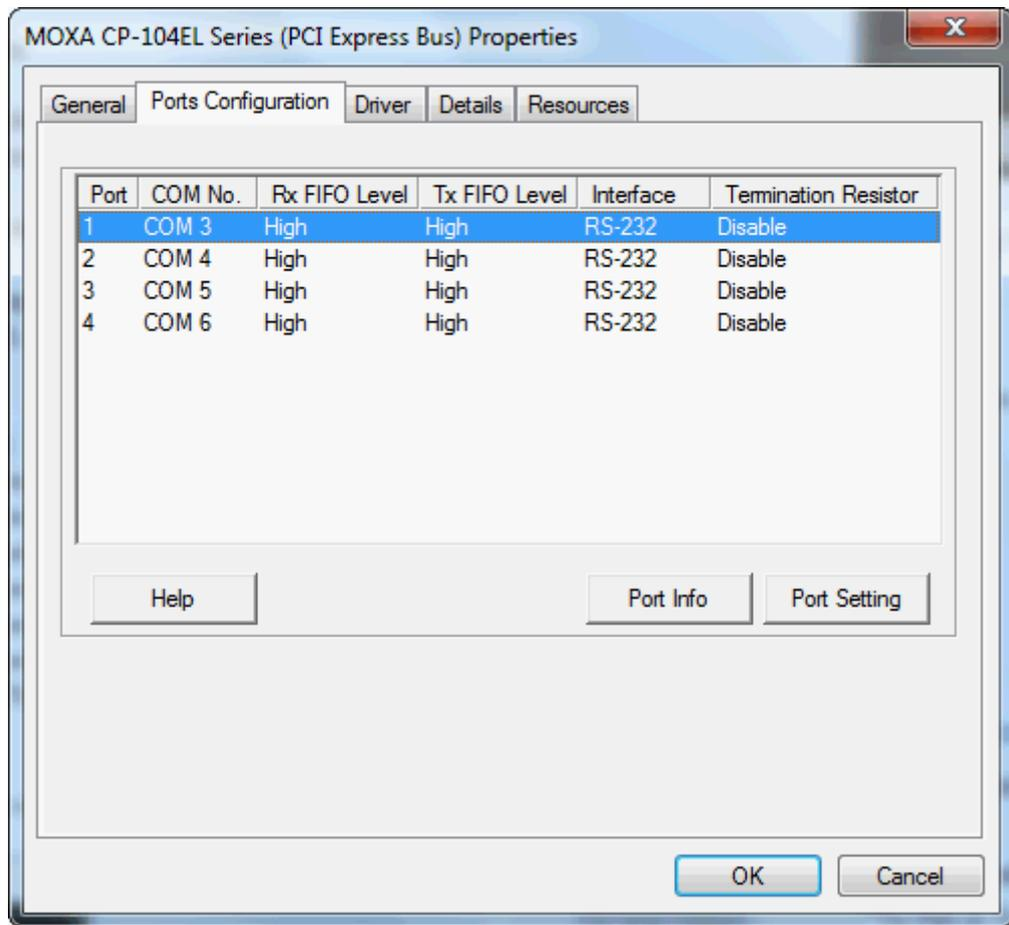
3. Select a COM number for the port from the **Port Number** pull-down list. Select the **Auto Enumerating COM Number** option to map subsequent ports automatically. The port numbers will be assigned in sequence. For example, if COM 3 is assigned to Port 1, then COM 4 (if not already occupied) will be assigned to Port 2, etc.
