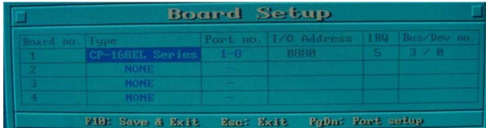
4. You may enter or modify the settings of each port at this stage. The values displayed first are the port's initial values that were set up when the driver was installed.
