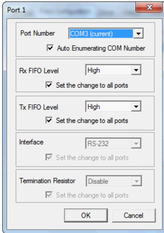
4. Select an **Rx FIFO Trigger** from the **Rx FIFO Level** pull-down list. Rx FIFO trigger levels of **High**, **Middle**, and **Low** are available, with the default set to High (120 bytes). Select **Set the change to all ports** option to apply this Rx FIFO Trigger to all ports.
