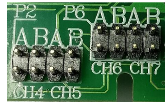
Thermocouple: Empty Pin A & B
