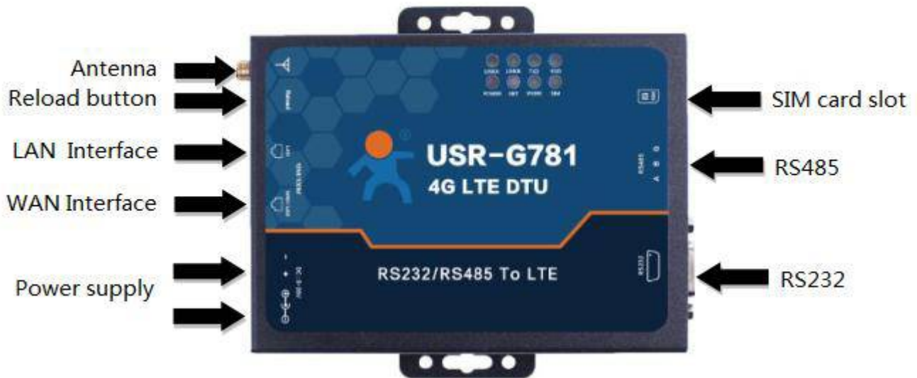
Figure 11 Hardware interface schematic diagram
