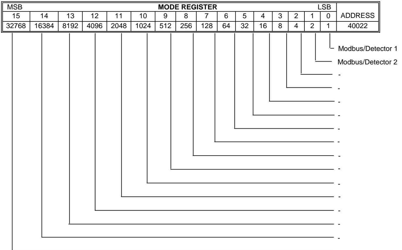
**Modbus/Detector Mode.** When this bit is set the relays will be connected to the Modbus register 40002. Relay 1 = bit 8, relay 2 = bit 9. When the bit is cleared then the relays will be connected to the detector.
