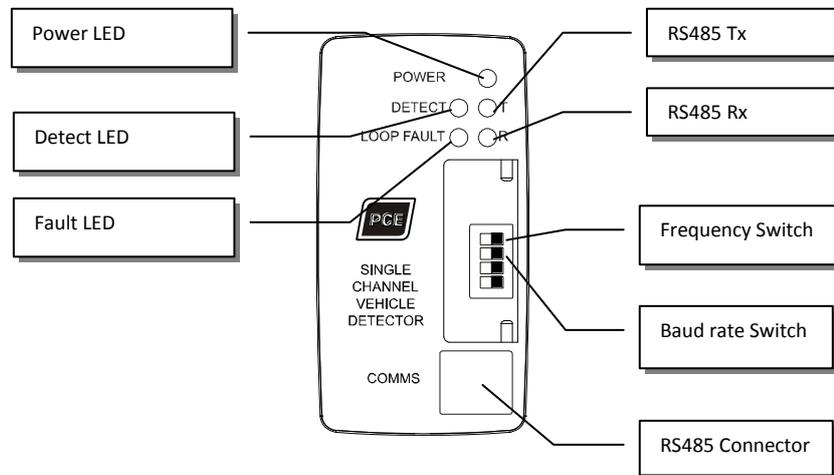
**Power LED.** Illuminates when the power is on.
