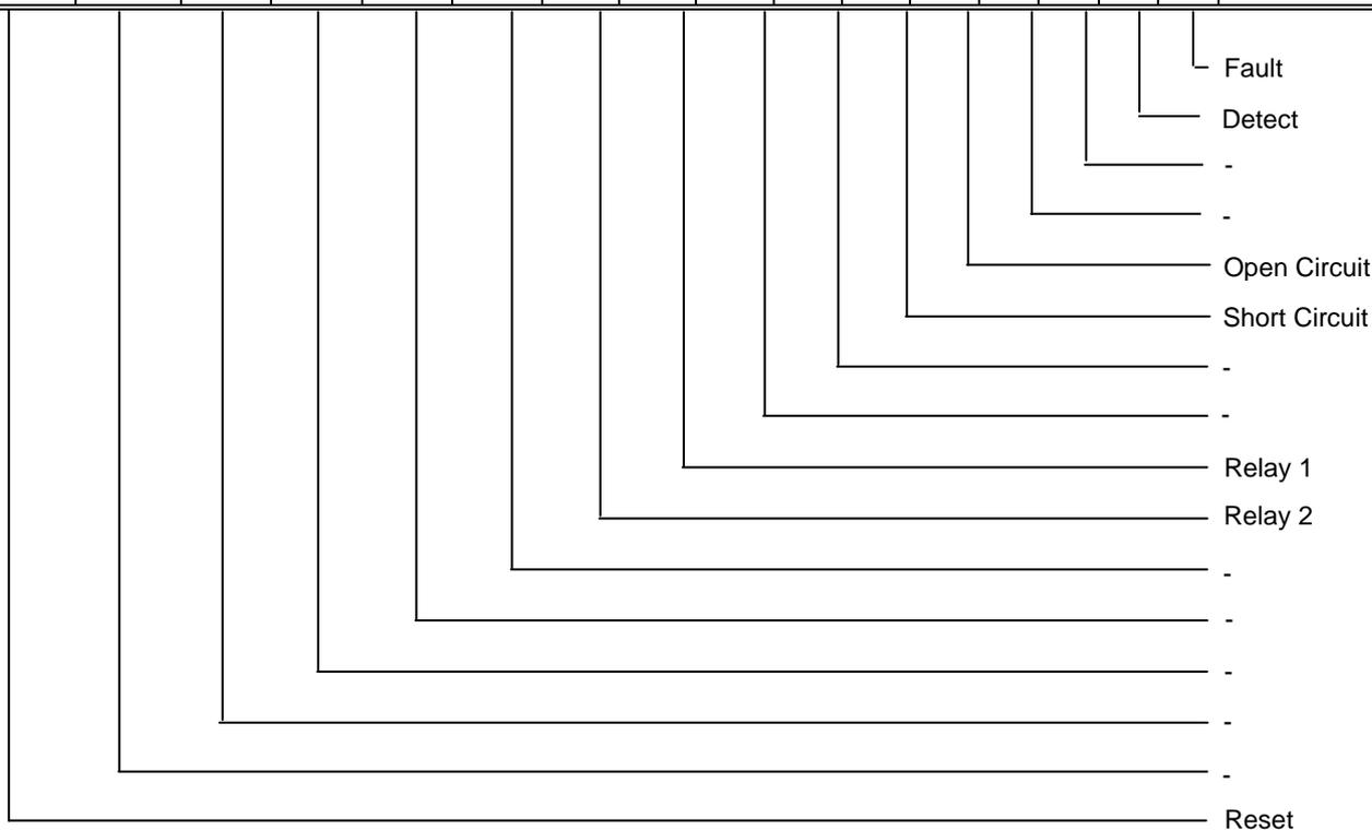
**Fault.** This bit will be set when there is a fault on the loop.
