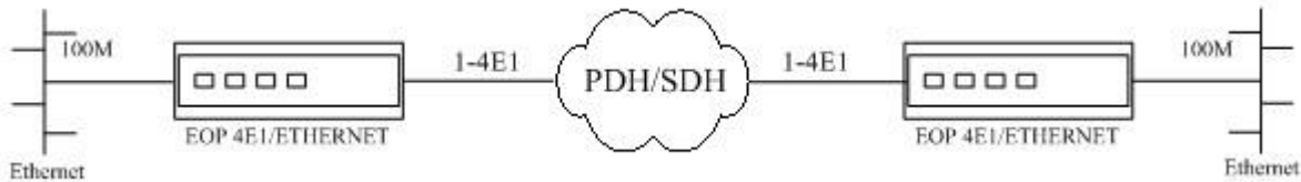
Figure 2-1 EOP 4E1 to Ethernet converter application
