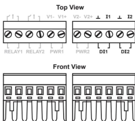
**STEP 1:** Insert the negative (ground)/positive DI wires into the  $\perp$ /I1 terminals.
