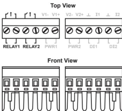
**FAULT:** The two sets of relay contacts of the 6-pin terminal block connector are used to detect user-configured events. The two wires attached to the Fault contacts form an open circuit when a user-configured event is triggered. If a user-configured event does not occur, the Fault circuit will be closed.
