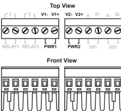
**STEP 1:** Insert the negative/positive DC wires into the V-/V+ terminals.
