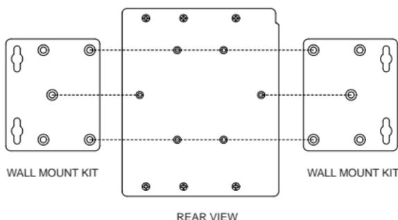
**STEP 2**—Mounting the EDS-600 on the wall requires 4 screws. Use the EDS-600, with wall mount plates attached, as a guide to mark the correct locations of the 4 screws. The heads of the screws should be less than 6.0 mm in diameter, and the shafts should be less than 3.5 mm in diameter, as shown in the figure at the right.
