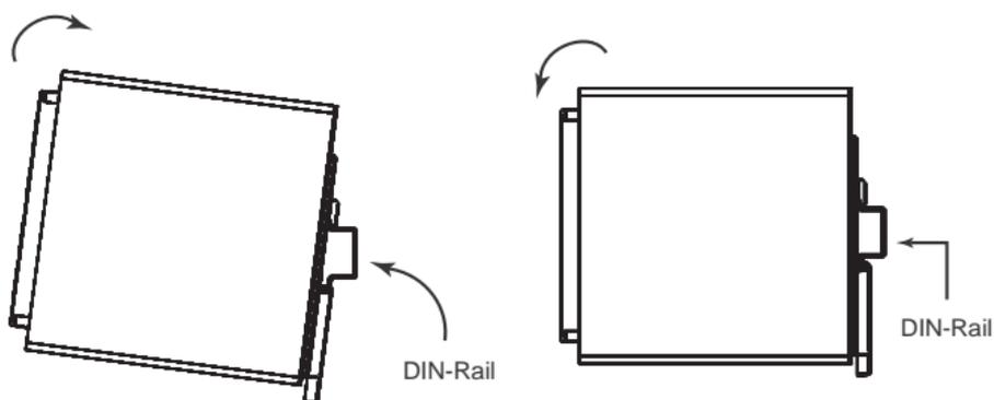
To remove the Moxa EDS-600 switch from the DIN-Rail, use a screwdriver to push down the spring-loaded bracket until it locks in place, as shown in the following diagram. Next, rotate the bottom of the switch upwards and then remove the switch from the DIN-Rail.
