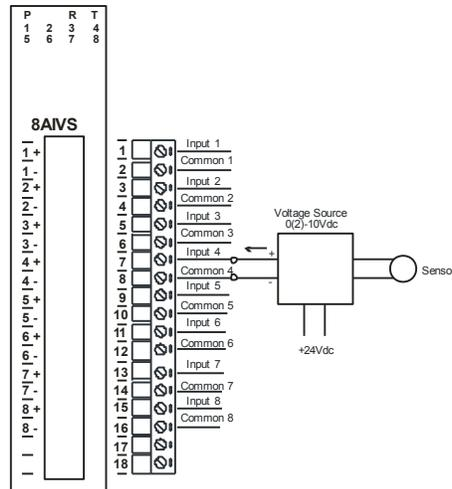
The following diagram shows the wiring for the power.
