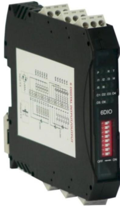
The outputs are written to by the Modbus master device such as a PC or PLC. Each output can be individually switched on or off, or all outputs can be set up at the same time by writing a single number to the output register which represents the status of all outputs.
