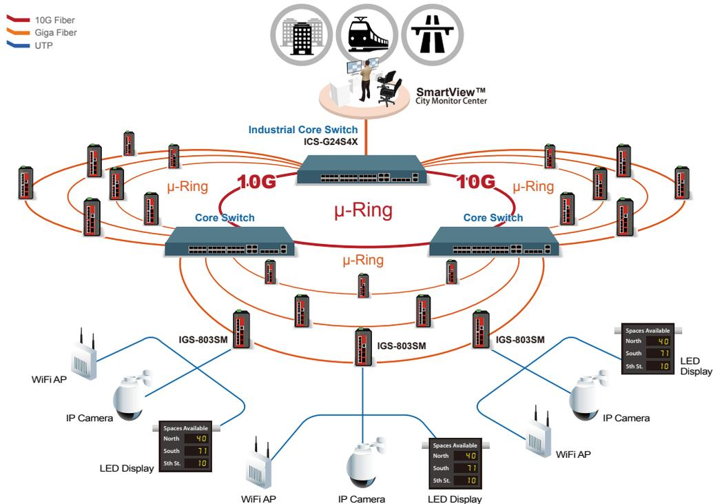
Figure 2 : 10G Backbone with μ-Ring topology
