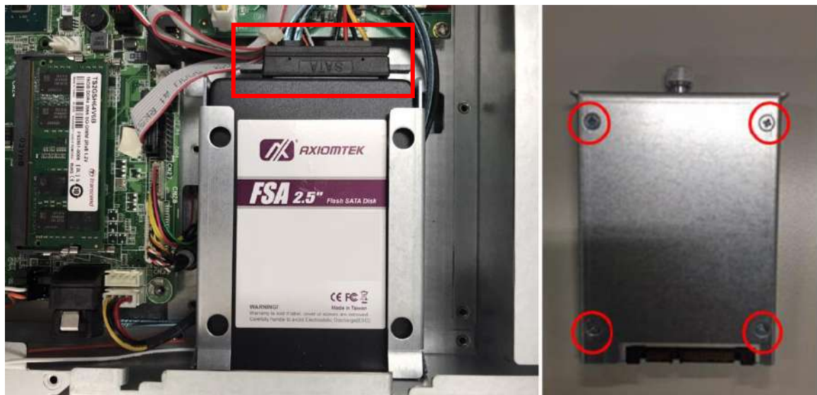
Figure 2-6 Fastening a HDD to the bracket and completing the installation
