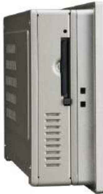
Figure 2.2 Install CFast Memory Card
