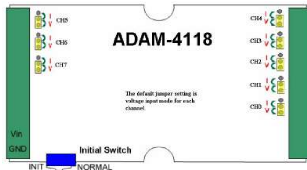
Figure 3.8 ADAM-4118-AE Jumper Settings
