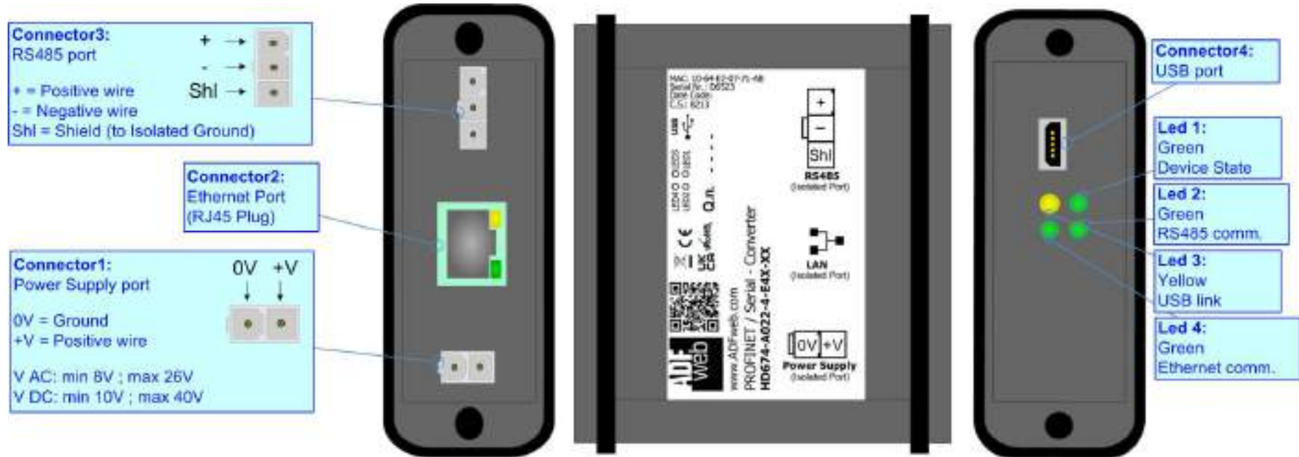
Figure 1c: Connection scheme for HD674-A022-4-E4x
