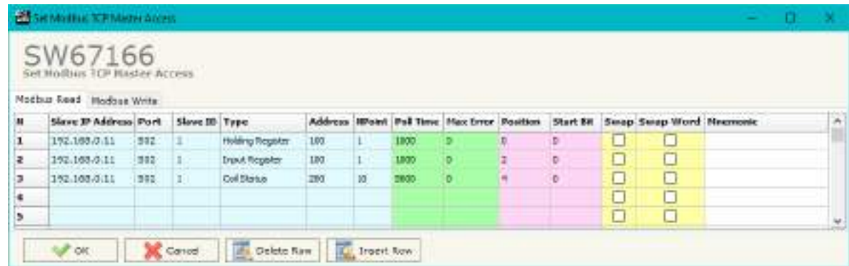
Figure 4a: "Set Access → Modbus Read"
