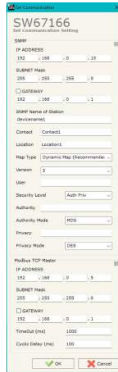
Figure 3: "Set Communication" window
