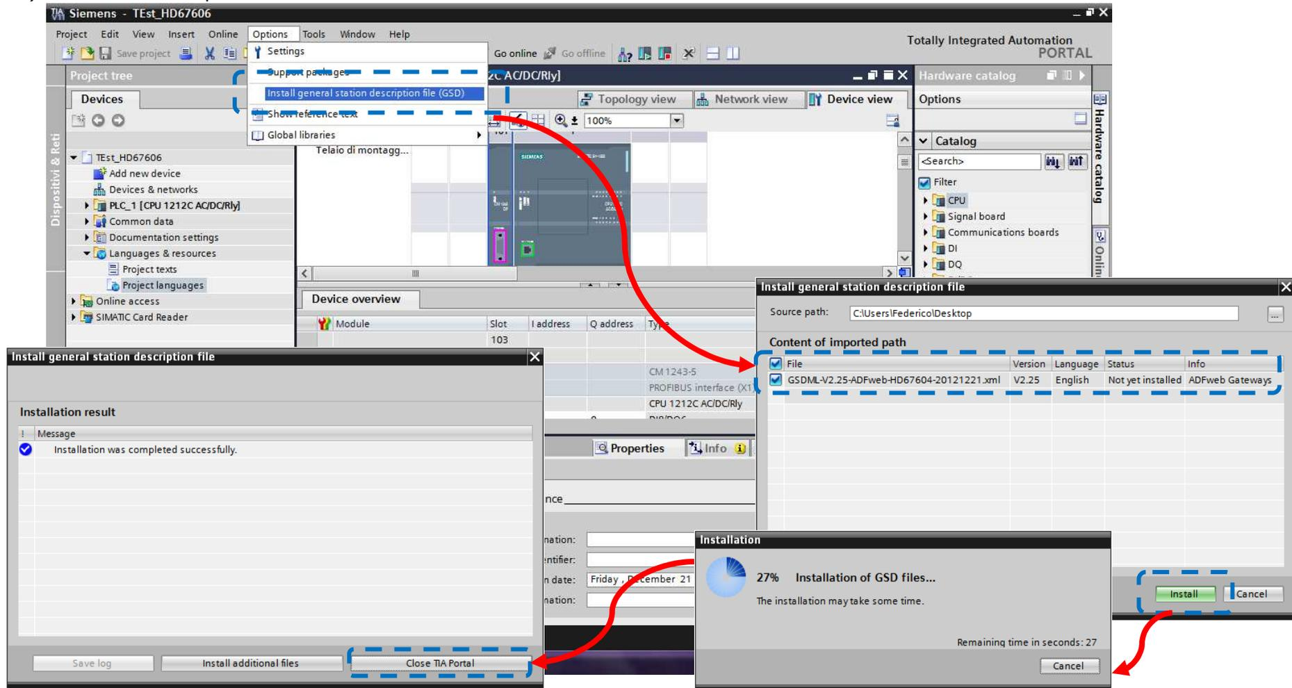
2) Import the module in the network; connect the device to the PLC network and edit the parameters of IP, station name etc.
