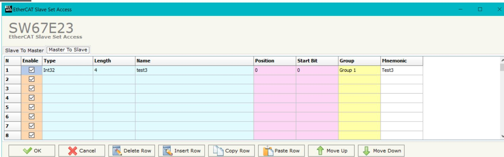
Figure 5b: "EtherCAT Slave Set Access → Master To Slave" window
