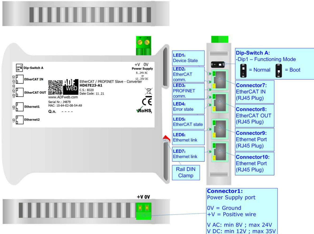
Figure 1: Connection scheme for HD67E23-A1
