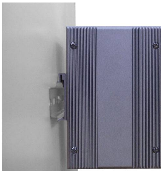
Figure 2.17 DIN-rail Step 2
