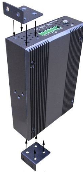
Figure 2.15 Combine the Metal Mounting Kit
