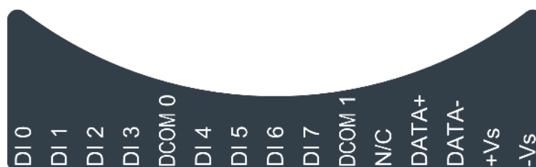
Figure 2.30 WISE-4051 Pin Assignment
