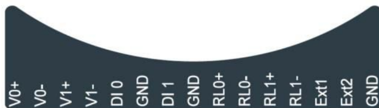
Figure 2.16 WISE-4012E Pin Assignment
