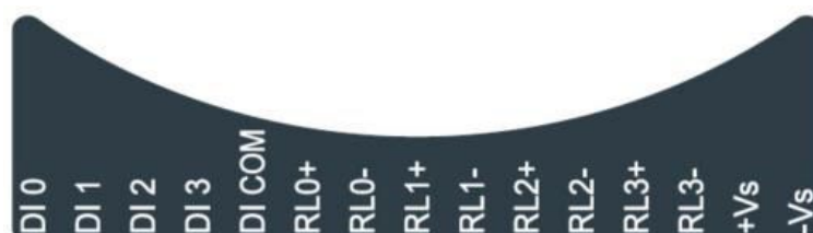
Figure 2.34 WISE-4060 Pin Assignment
