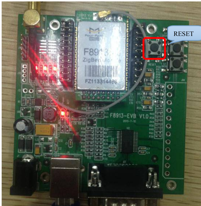
figure 2-9 The “reset” button on the development board
