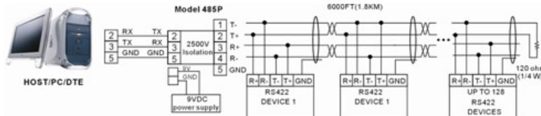
Figure 4: Master/Slave multi-drop configuration in RS422 mode
