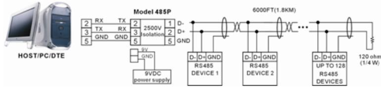
Figure 2: Master/Slave multi-drop configuration in RS485 mode
