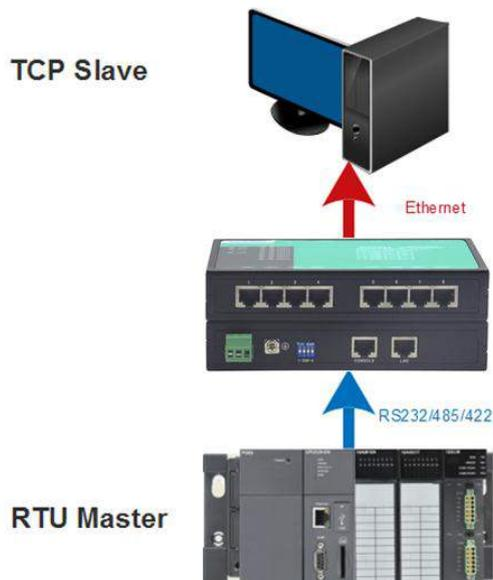
In RTU Master Mode, the RTU master device accesses the TCP slave device through the gateway.
