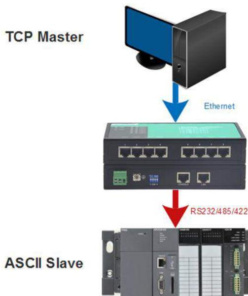
In ASCII Slave Mode, the TCP master device accesses the ASCII slave device through the gateway.
