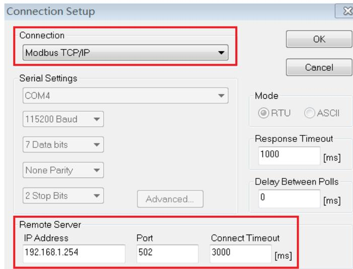
14. In the "Remote Server" check box, configure the Modbus gateway IP address, port number, and connection timeout.
