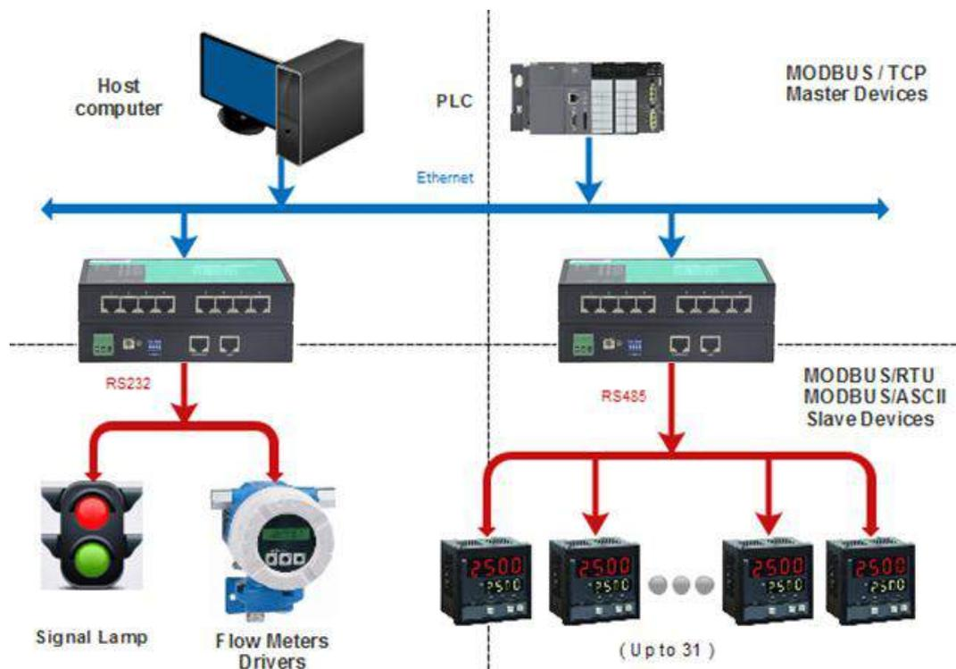
In RTU Slave Mode, the TCP master device accesses the RTU slave device through the gateway.
