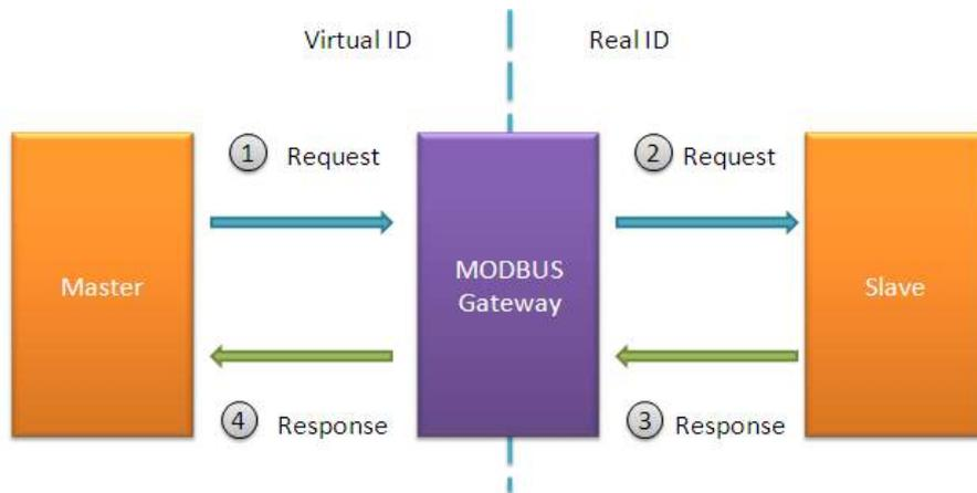
The gateway implements the function of ID mapping by setting the ID range and the ID offset. The ID range starts from the slave start ID to the slave end ID. Only channels with channel type slaves can be mapped, including serial port (RTU Slave or ASCII Slave) and TCP Slave.
