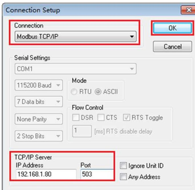
6. Enter the TCP slave IP address "192.168.1.80" in the "IP Address" text box of the "TCP / IP Server" area.
