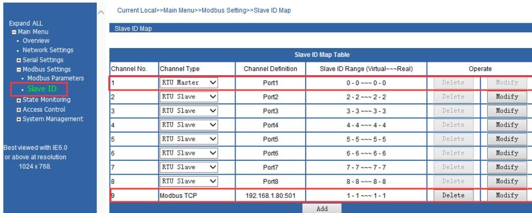
2. In the "Channel NO." is 1, click the "channel Type" drop-down list box and select "RTU Master".
