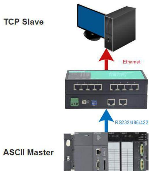
In ASCII Master Mode, the ASCII master device accesses the TCP slave device through the gateway.
