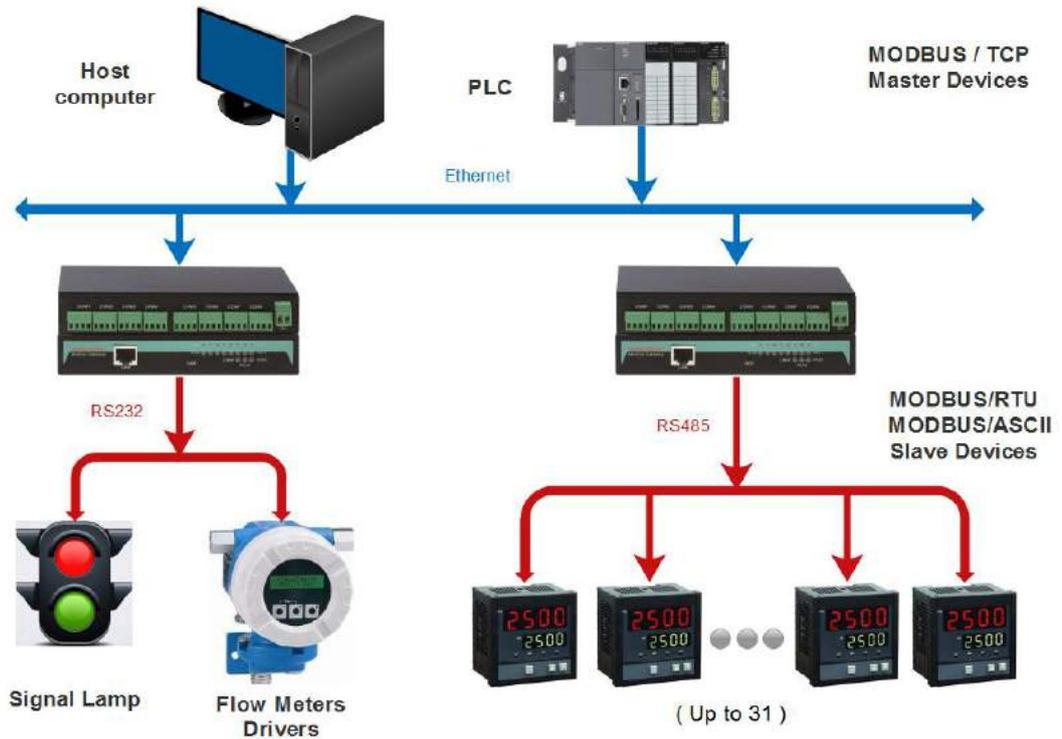
Modbus Basic Architecture Figure is shown below:
