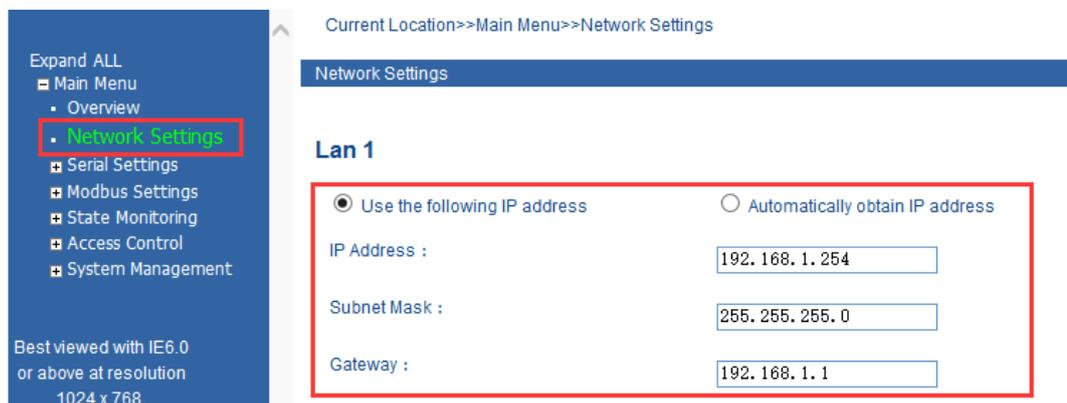
1. Log in to the Web configuration interface and select "Network Setting".
