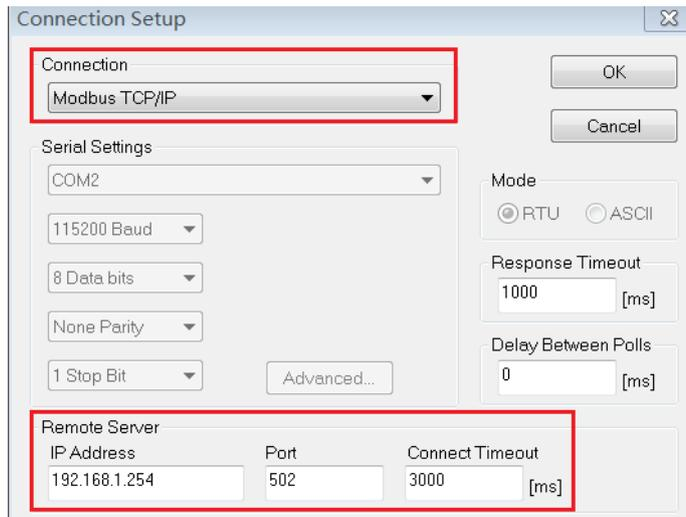
14. In the “Remote Server” check box, configure the Modbus gateway IP address, port number, and connection timeout.
