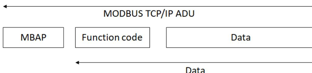
Use a special message header on TCP / IP to identify the Modbus application data unit. This header is called the MBAP header (Modbus protocol header).
