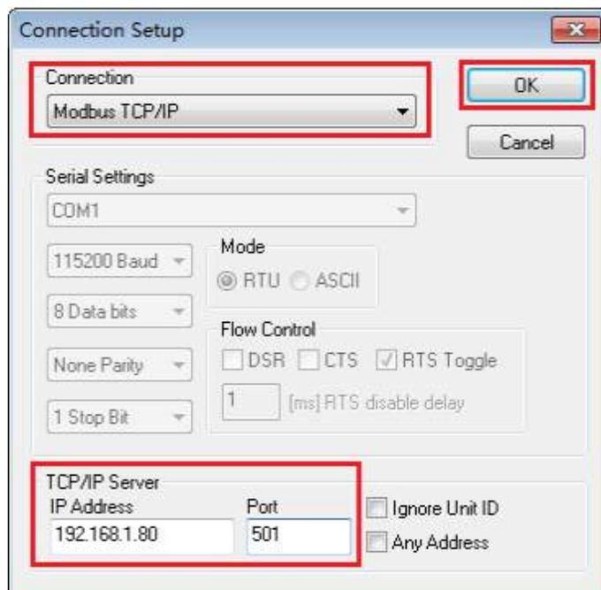
6. Enter the TCP slave IP address "192.168.1.80" in the "IP Address" text box of the "TCP / IP Server" area.
