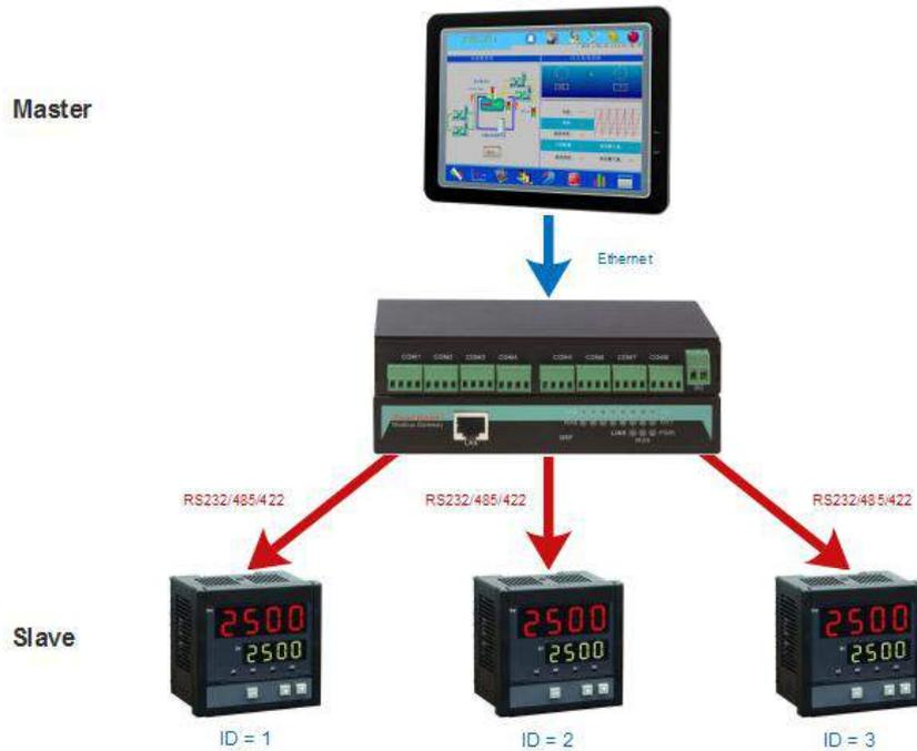
**Use TCP Master instead of serial port master, do not change the original device Slave ID**
