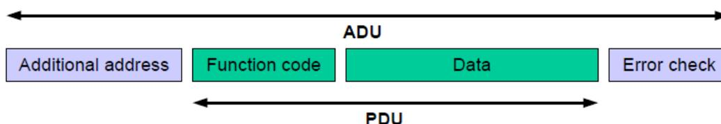
The Modbus application data unit is built by the client that initiates a Modbus transaction. The function indicates to the server what kind of action to perform.
