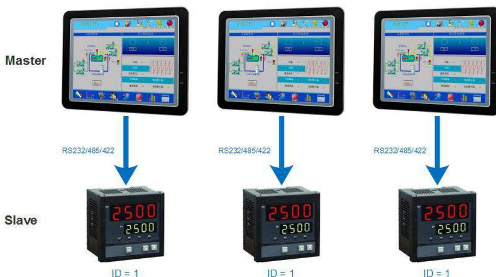
The new system using the Modbus gateway is connected to each of the serial Slave devices, so the Ethernet SCADA can control them. But Slave ID in the network cannot be duplicated, so some devices need to change the ID so that the network can identify them.
